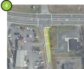
4 Dillard Rd. - new right turn lane (est. $555,000)
